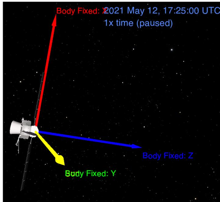
The asymmetrical spacecraft is subject to a torque produced by the solar radiation pressure. The flight rules impose that the body-fixed Y-axis must be at maximum 1 arcsec from the spacecraft-Sun direction. At the beginning the spacecraft has an offset angle of +3 arcsec along the body-fixed X-axis and is not rotating. The new control law must bring the attitude back inside the 1 arcsec threshold in no more than 30 s.
